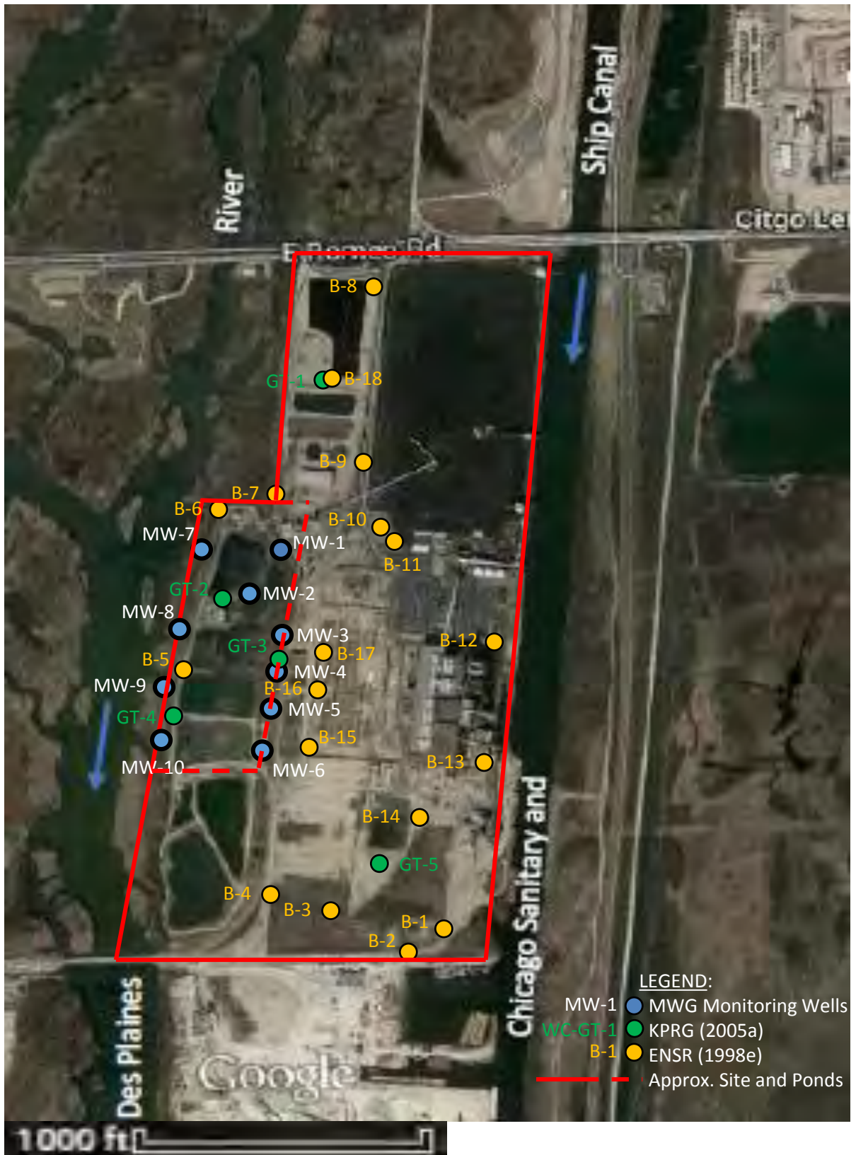
Figure 4 Will County Soil Boring Locations (PCB 2013-015)
